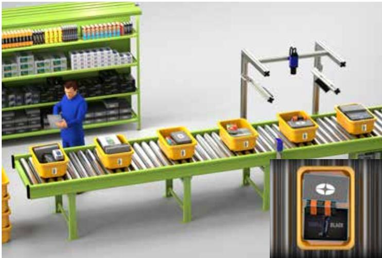
Datalogic vision systems running the IMPACT Pattern Sortation Tool enable countless machine vision applications for pattern recognition. The Pattern Sorting tool enables cross-check applications that ensure package contents match the information on the pallet or tote label.
