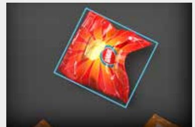
IMPACT Pattern Sorting Tool identifies and locates objects even in soft packaging such as chips, biscuits, frozen goods and pasta, enabling robot picking and sorting.
