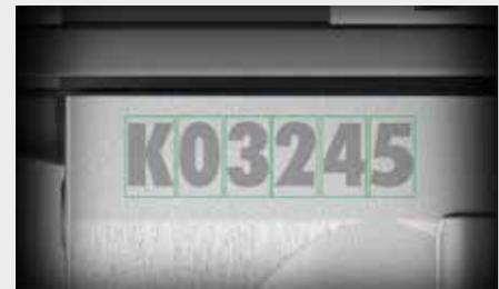
The outstanding Advanced OCR software algorithm ensures the highest reading reliability of ink-jet dot matrix characters on challenging surfaces (i.e. cans, bottles,..)
